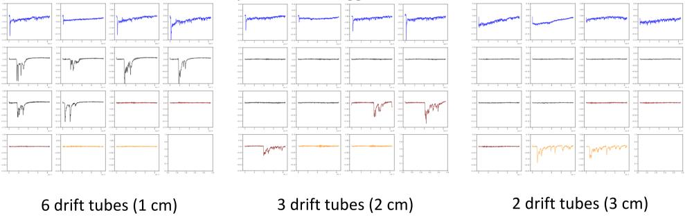
vertical full scale 300 mV (gain 10) – horizontal scale 800 ns
