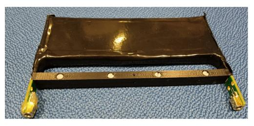
16 channels data acquisition board designed and used by the MEG2 experiment at PSI ( $\mu \rightarrow e + \gamma$ ) (credit to S. Ritt, Paul Sherrer Institute, Zurich, Switzerland) 12cm x 6cm upstream and downstream scintillator tiles (designed and used as timing counter of the MEG2 experiment at PSI) used in coincidence and readout by SiPM
