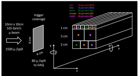
The test was performed during November 2021 at CERN on the H8 beam line in a **parasitic mode**. Main users on the same beam line was a team testing a tile calorimeter and, therefore, requesting for **large part of the time, beams of electrons and hadrons, at various energies,** needed for their calibration, but **useless for our purposes**. Only **sporadically**, a beam of **165 GeV/c muons** was available for us.
