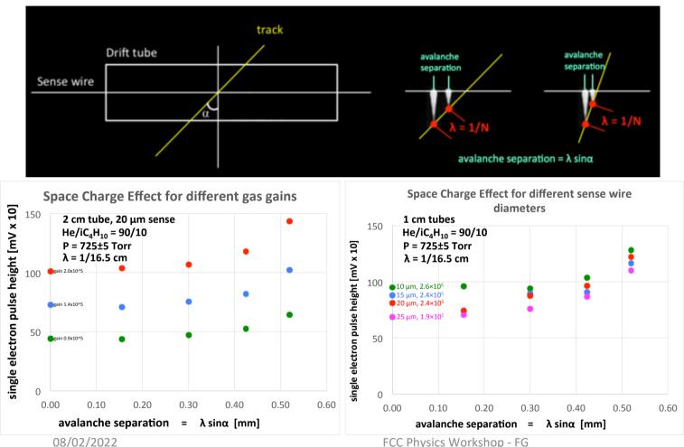
no dependence of space charge effects from the gas gain, no dependence of space charge effects from the sense wire diameter at least in this range of gas gain values
