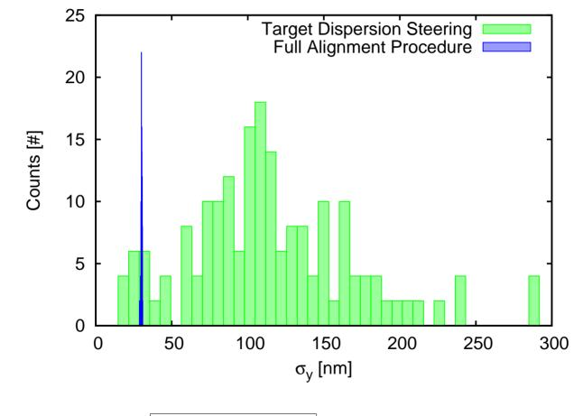
$\Rightarrow$  Final vertical beamsize is  $\sigma_y = (30.0 \pm 0.3)$  nm (AS BAD AS BEFORE!)
