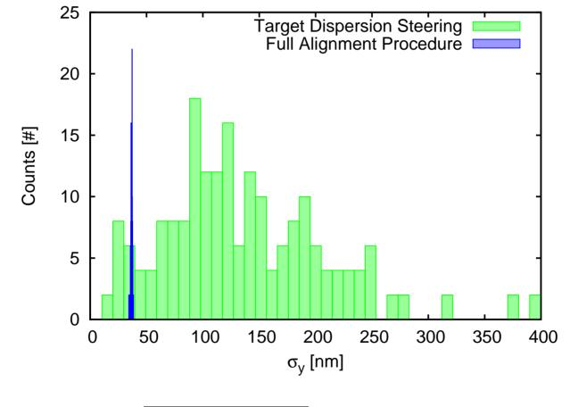
$\Rightarrow$  Final vertical beamsize is  $\sigma_y = (36.7 \pm 0.6)$  nm (AS BAD AS w/SR!!)
