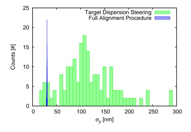
$\Rightarrow$  Final vertical beamsize is  $\left| \ \sigma_y = (30.0 \pm 0.3) \ {\rm nm} \right.$
