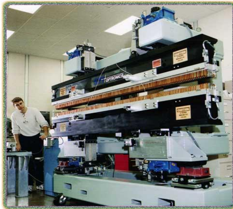
Undulator Insertion Device at the Advanced Photon Source (USA)
