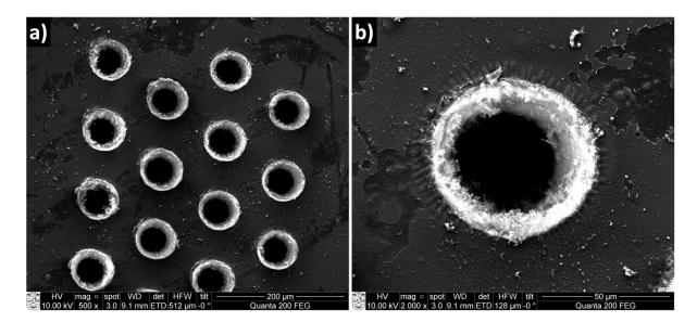
SEM micrographs of holes formed in **KAPTON coated with DLC**: a) small fraction of hole array formed by removing DLC prior to drilling, b) a single hole from the array, showing DLC crumpling KAPTON average hole diameters:
