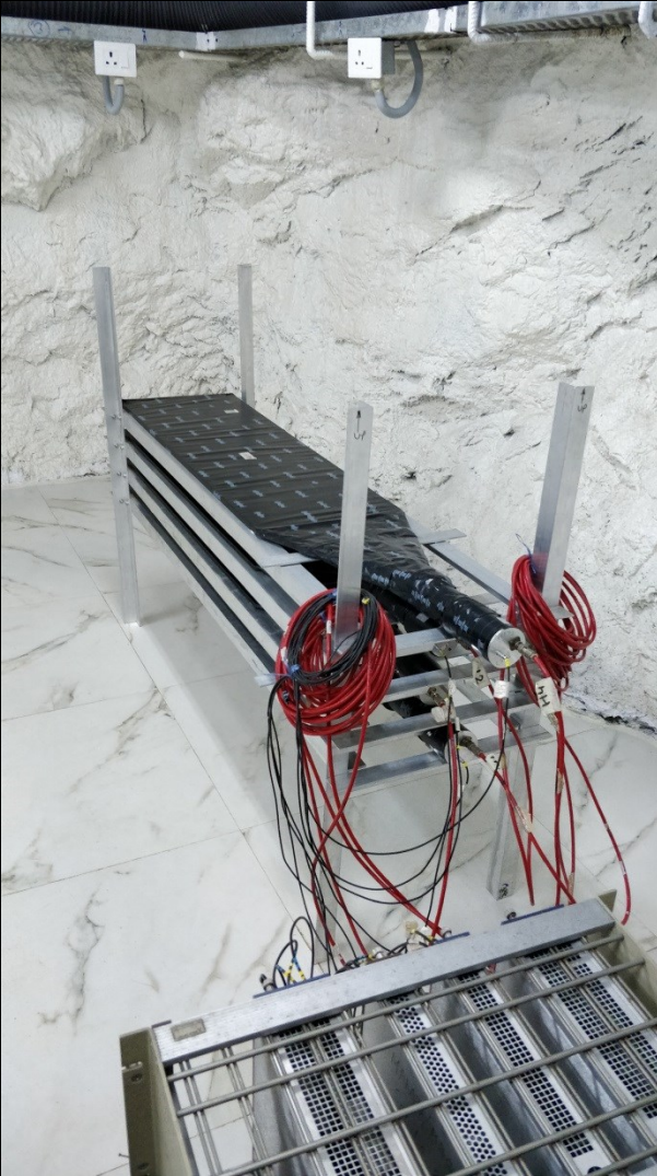
Muon Flux measurements using 4-fold coincidence
