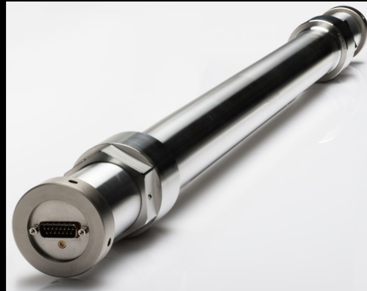
Neutron background measurements with combined fast and thermal neutron detectors
