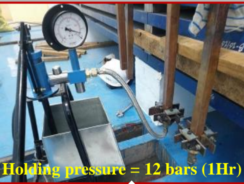
Coil Hydrostatic Pressure test
