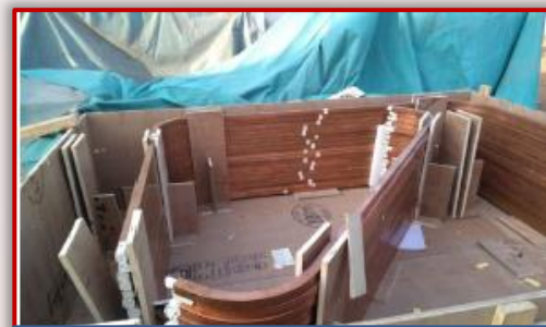
2 coils, 18 turns each X-sec 30 X 30 mm 2 and 17 mm bore
