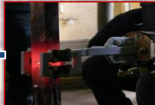
Induction brazing in progress
