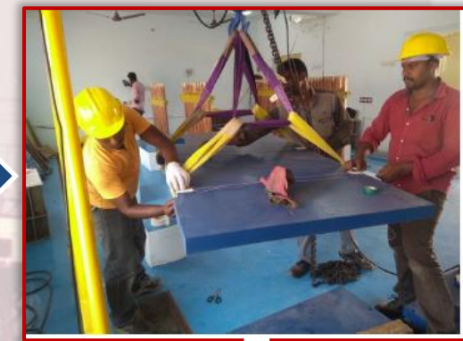
Iron plate lifting using gantry
