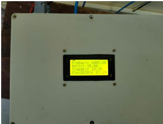
Instrument to monitor ambient parameter and flow rate (built in-house)
