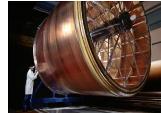
Time Projection Chamber (ALICE Experiment)
