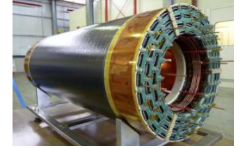
Cylindrical GEM detector (KLOE-2 Experiment)
