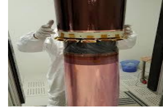
Cylindrical GEM detector (BES III Experiment)
