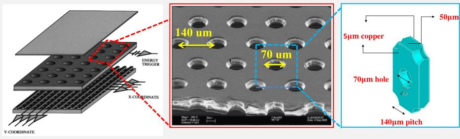
Fabio Sauli, The gas electron multiplier (GEM): Operating principles and applications, Nuclear Instruments and Methods in Physics Research A 805 (2016) 2-24
