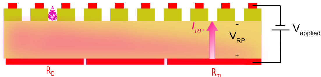
Fig: Charge deposited at a point evacuates to anode through the volume of resistive plate. This has an effect at other regions also.
