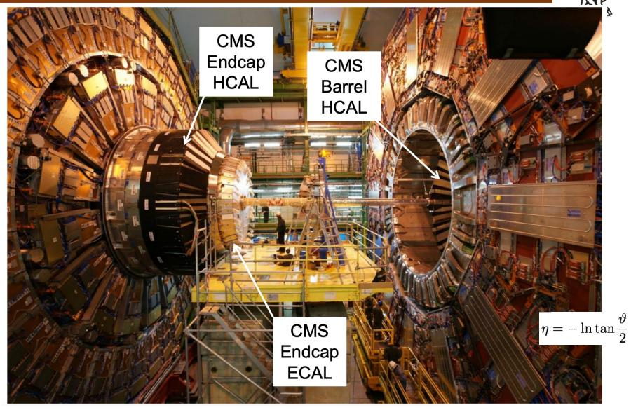
Sampling calorimeter with hermetic coverage
