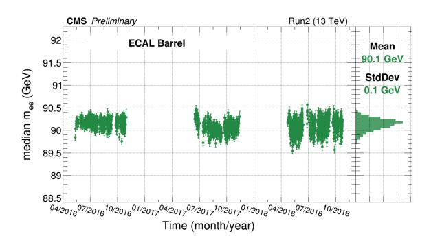
Time stability of the di-electron invariant mass distribution for the full Run2 data-taking period using Z→ee
