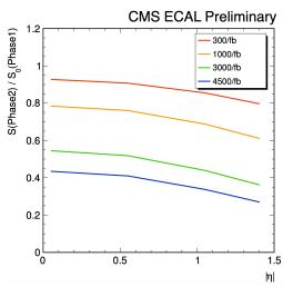
Expected signal loss in EB (0  $\leq$  | $\eta$ | < 1.5) from 55% to 70% at 3000 fb<sup>-1</sup>
