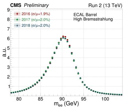
Invariant mass distribution comparing 2016, 2017, and 2018 data-taking period using Z→ee events with a refined re-calibration performed in 2019 for the full Run2 dataset.
