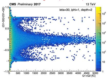
Good separation can be observed between particles directly hitting the PMTs sitting at low time values, and hits from standard collision particles
