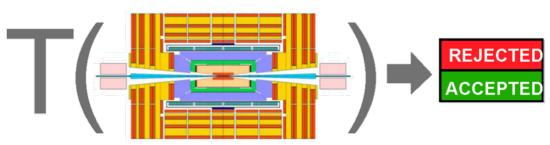
L1 Trigger receives simplified detector information from calorimeters and muon systems, and forms
