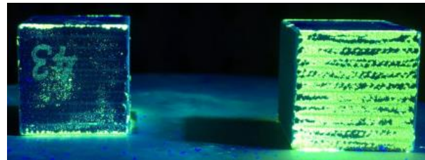
Comparison of an virgin sample (left) and a sample after loading (right) under UV light prior application of a fluorescent penetrant.
