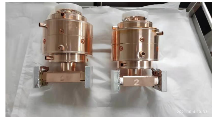
1 st and 2 nd stage storage cavity
