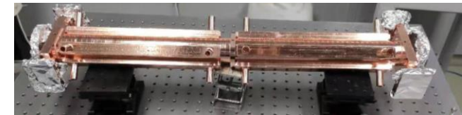
X-band 72 cell structure
