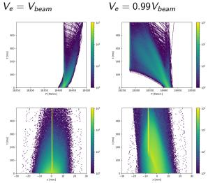
Evolution of momentum distrubition and horizontal distribution of ion beam in simulation of cooling with dispersion and space charge of electrons for two different mean electron velocities.
