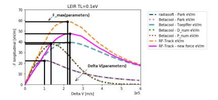
Value of maximum force or  $\Delta V$  for it for particular set of parameters.  $\downarrow$ Value of maximum force or  $\Delta V$  for it for scanning over one choosen parameter.
