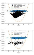
Comparison of input ion beam  $V_z(x)$  distribution with the beam after 200ms and 500ms of cooling simulation.
