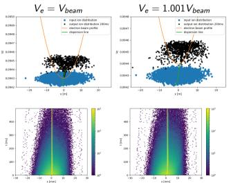
Comparison of input ion beam  $V_z(x)$  distribution with the beam after 200ms of cooling simulation.
