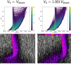
Evolution of momentum distribution of ion beam in a simulation of cooling with dispersion and space charge of electrons for two different mean electron velocities. Dispersion:  $D_x=1m$ ,  $D_y=0m$
