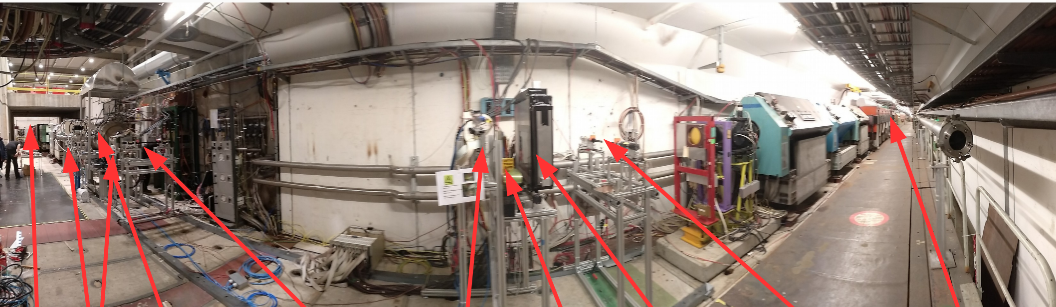
COMPASS 4 x silicon (DUT) High-pressure H TPC (DUT) Trigger scintillator Silicon (DUT) VMM GEM (DUT) SciFi station Trigger scintillator M2 beam
