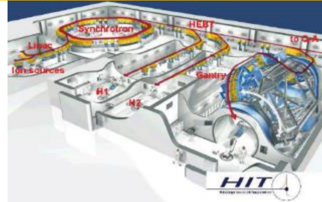
Layout of the Heidelberg Ion Therapy facility
