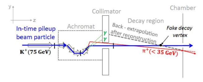
K<sup>+</sup> decay/interaction in the achromat Photons blocked by the collimators
