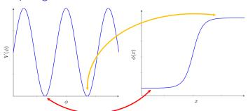
A static soliton "kink" solution of the classical equation of motion in the Sine-Gordon model:
