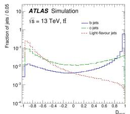
Tracking & jet information condensed using multivariate (MV) algorithms for separation of b-jets vs different flavour jets - c or light-flavour
