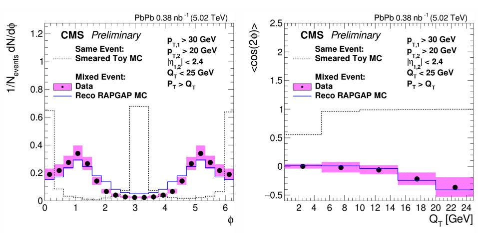
**Toy MC**: back-to-back jets with detector resolution effects  $\langle \cos(2\phi) \rangle \to 1$  Mixed events have only acceptance affects and have  $\langle \cos(2\phi) \rangle$  negative
