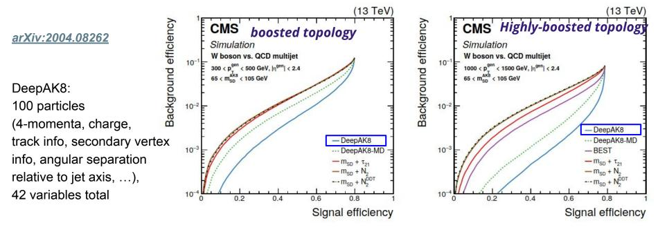
Performance of taggers & scale factors is highly sensitive to modeling of quark- and gluon-initiated jet parton showers. Important to have as many experimental inputs to constrain these uncertainties!!
