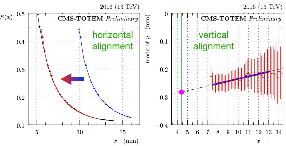
Detector alignment is performed in various steps
