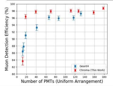
Left: Tagging efficiency with uniform PMT distribution (98% reflectivity, 200 ns window)
