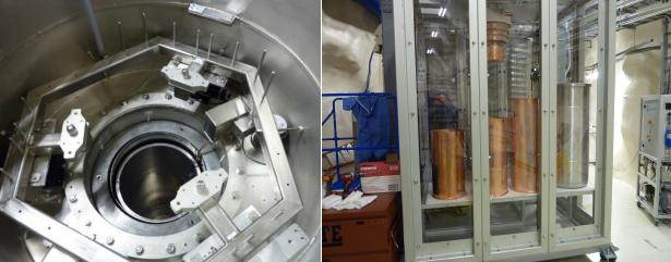
CUTE drywell: suspension system and shielding CUTE cryostat open inside the CUTE cleanroom layers
