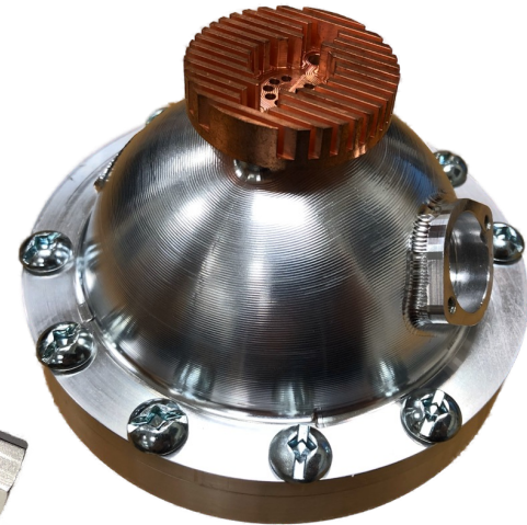
Examples of Integrating Spheres used at Prof. A. Meldrum's Lab at UofA (images via W. Morrish )
