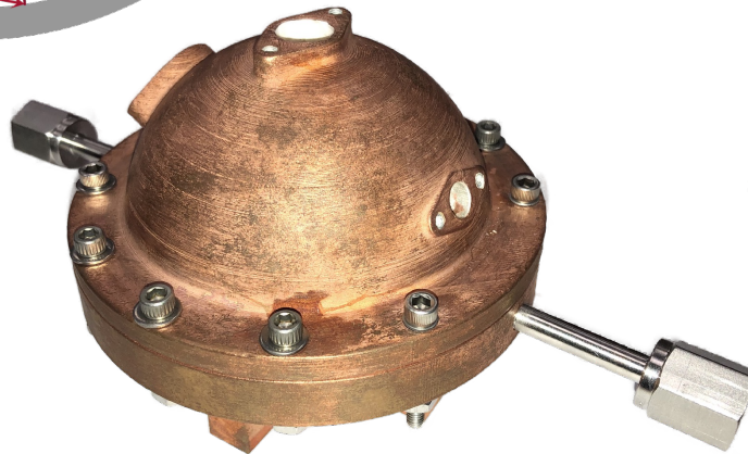
Examples of Integrating Spheres used at Prof. A. Meldrum's Lab at UofA (images via W. Morrish )
