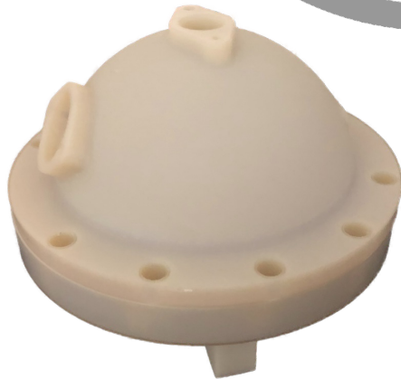
Examples of Integrating Spheres used at Prof. A. Meldrum's Lab at UofA (images via W. Morrish )
