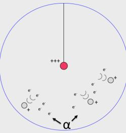
There is <sup>210</sup>Po contamination in the copper surface, which causes alphas that ionize a lot of gas. All the ions create a space charge that disturbs the electric field, and changes the electron drift time. For some still unknown reason, a high rate of low energy events keep happening for around 5s after each alpha.
