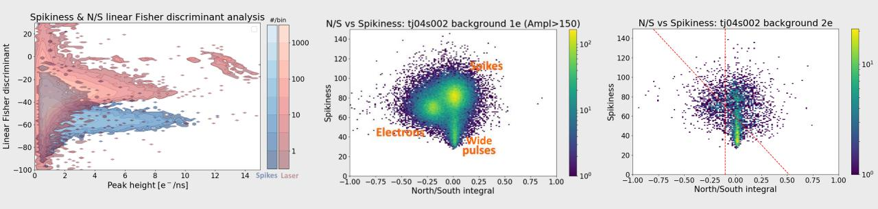
The separation between electron and spike events is weaker at lower energies. Wide pulses are another dominant background of unknown origin in the data. A cut on N/S removes fat pulses (dominant in 2-peak data) and a Fisher discrim. cut removes spikes.
