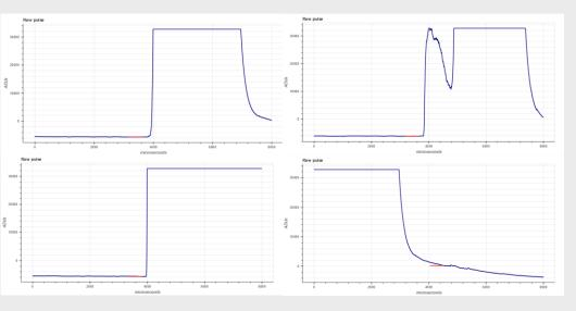
The saturated alpha signals can be broken up and difficult to detect, but using the drift time, rate of events and decreasing baselines, we can identify alphas and remove most of the low-energy background due to them with a 5s cut after each alpha, keeping 85-90% of the total time.
