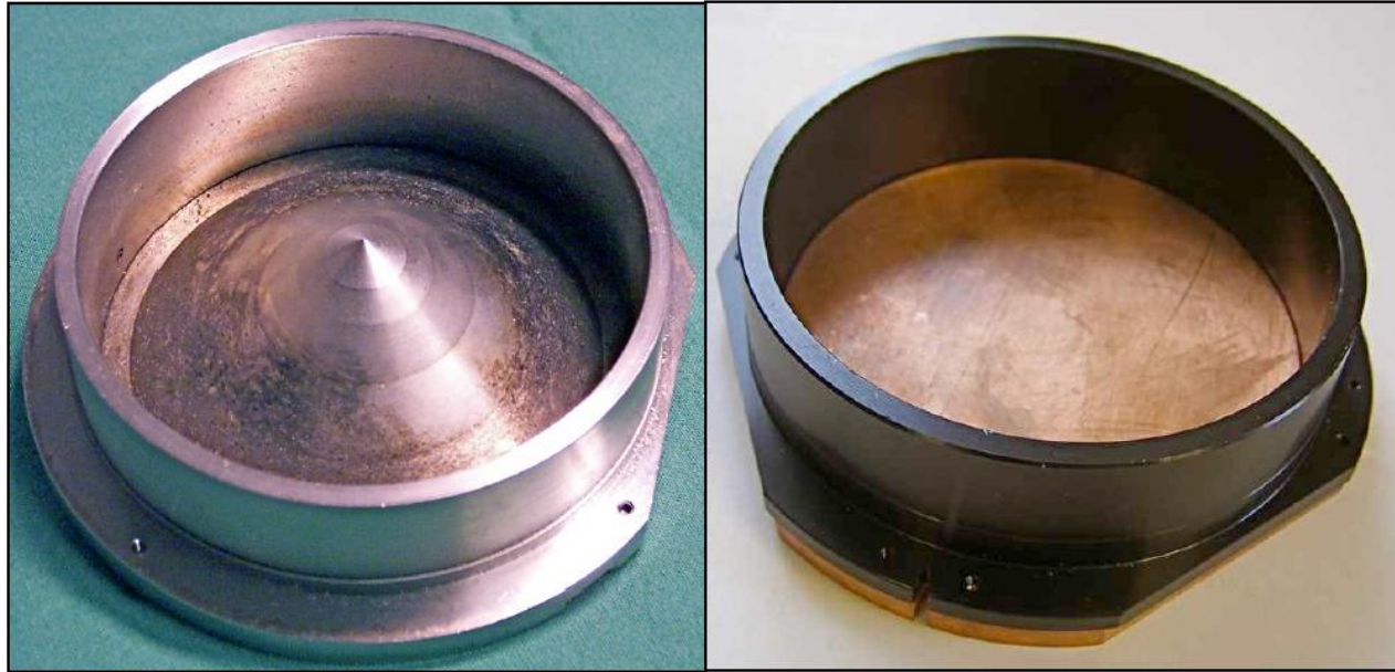
Figure 2.1 A conventional flattening filter for a 6 MV beam (left) and the copper plate used in the flattening filter free mode (right).
