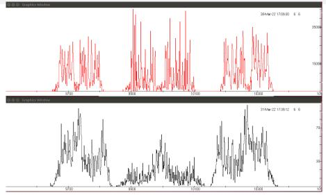
$\bullet$  Simulation is red. This would give the wider  $\gamma\text{-ray}$  peak than exp.
