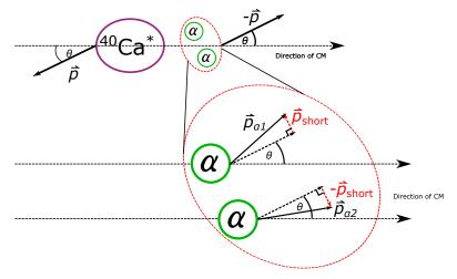
• Parameters  $\theta$  and  $p_{short}$  :  $p_{\alpha i}$  ratio make the model flexible.
