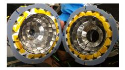
Allows to identify products of fusion evaporation raction while suppressing other reaction channels like Coulomb excitation or elastic scattering.
