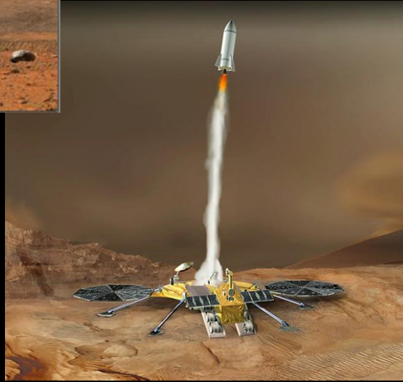
Mars Ascent Vehicle (MAV) launches Orbiting Sample (OS)
