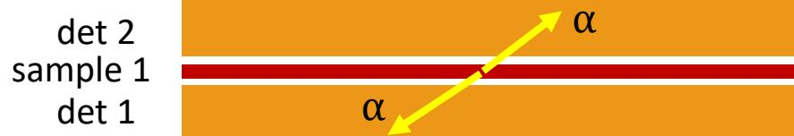
Silicon detectors in the neutron beam
