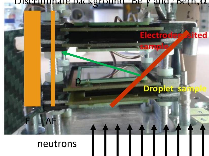
Silicon detectors OFF the neutron beam
