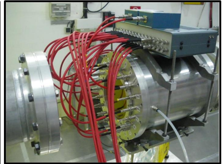
MGAS@n\_TOF ==> Beam monitoring with  $^{10}B(n,\alpha) + \sigma$  of  $^{14}N(n,p)$ ,  $^{33}S(n,\alpha)$ ,  $^{35}Cl(n,p)$
