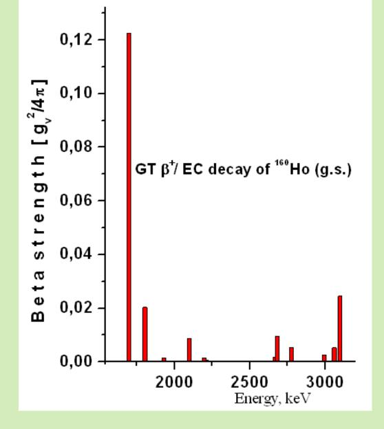
$S_{\beta}(E)$  for Gamow–Teller transitions in the  $\beta$ +/EC decay of the deformed nucleus <sup>160g</sup>Ho (5+;25.6 min),  $Q_{EC}$  = 3286(15) keV.
