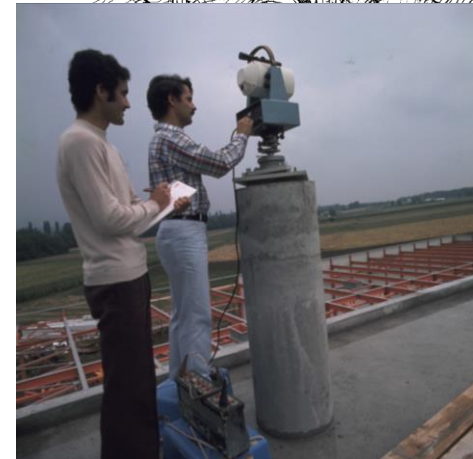
Distance measurement with a MA 100 tellurometer
