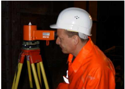
Nadir plumb instrument
