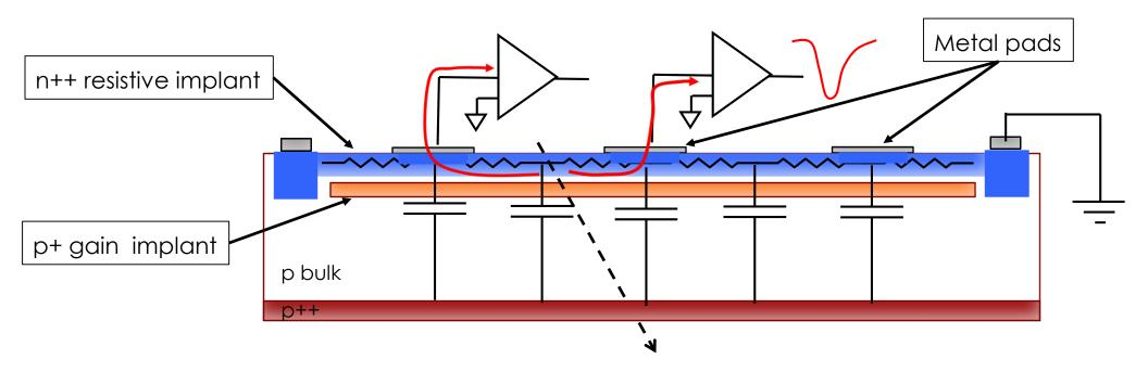
In this design, the charges collected on the n++ flow to the electronics as in standard sensors The read-out pads are embedded into a resistive n++ sheet that assures pad isolation
