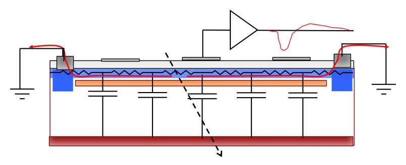
In this design, there is only 1 contact to the n++: the charges collected on the n++ flow to the edge of the sensor.
