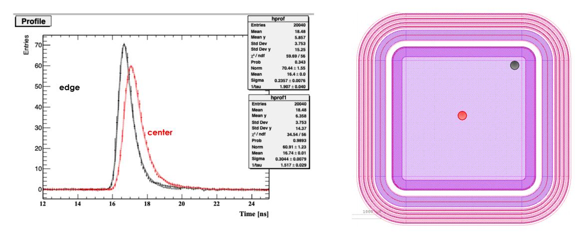
Even after a sizable distance,  $\sim 1$  mm, the rising edge is still quite sharp The signal shape is that of an exponetially modified gaussian
