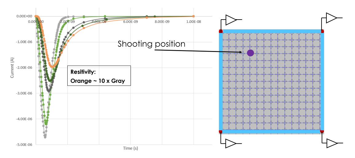
As the n++ resistivity increases, the simulation predicts shorter and wider signals
