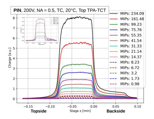
Charge collection measurement in a PIN:
