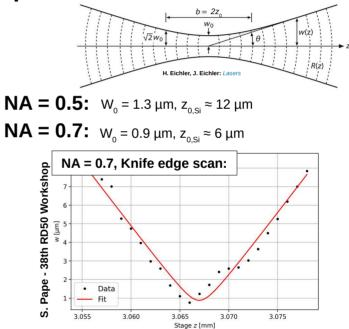
Rayleigh length for NA = 0.7 is approx. two times smaller  $\rightarrow$  Volume of charge generation along the beam axis by a factor of two smaller
