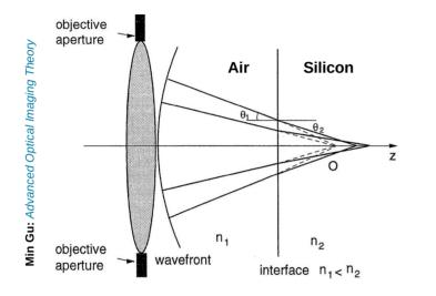
**Aberration:** light rays of different incident angles are focused at different positions on the axis
