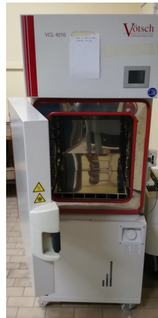
Vötsch VCL4010 Test Chamber with temperature range from -40 to +180°C available in Torino Laboratory
