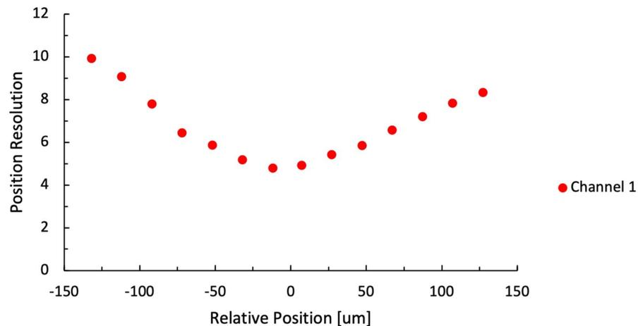
$$\text{Position Resolution } \sigma(\text{Pos}) = \sqrt{2} \frac{d(\text{Position})}{d(\text{Fraction})} / \left(\frac{S}{N}\right)$$
