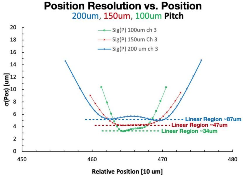
This plot is the position resolution plot for the BNL strips based on data taken by the FNAL beam test.
