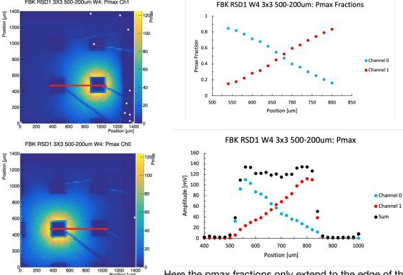
Here the pmax fractions only extend to the edge of the metal pad
