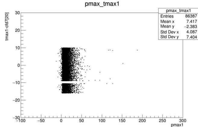
In Tmax vs Pmax scatter plots, Tmax corresponds to the time that the pulse reached its maximum value, and pmax corresponds to the maximum value of the pulse.
