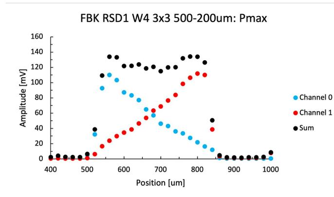
Here the pmax fractions only extend to the edge of the metal pad
