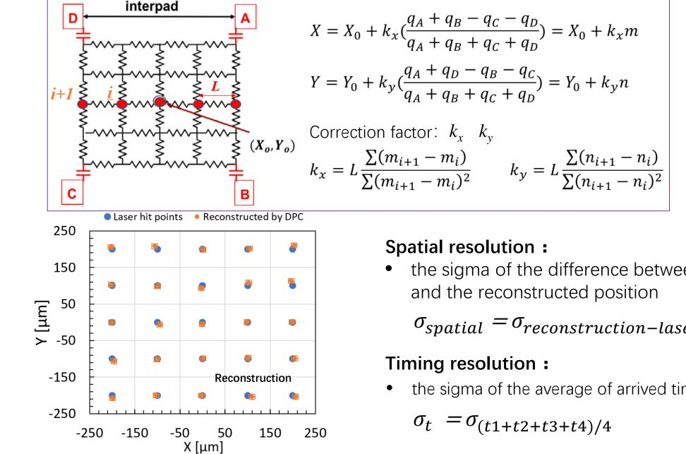
Discretized Positioning **Circuit model** (DPC)
