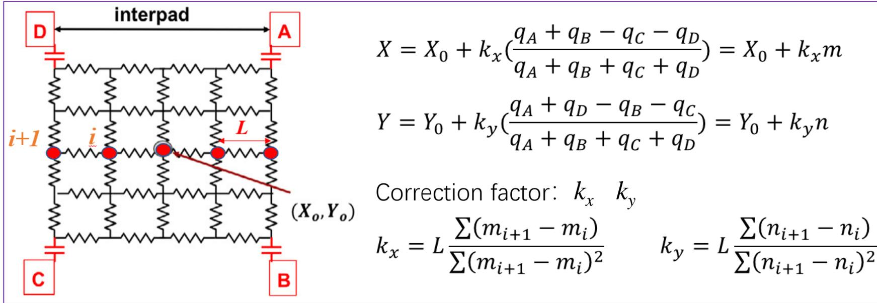
**Discretized Positioning Circuit model (DPC)**
