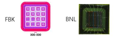
According to the current report, the pitch size of AC-LGAD is 50~500 µm, such as FBK / BNL AC-LGAD <u>https://indico.cern.ch/event/861104/contributions/4503072/attachments/2306</u> 673/3924214/H.%20Sadrozinski.pdf
