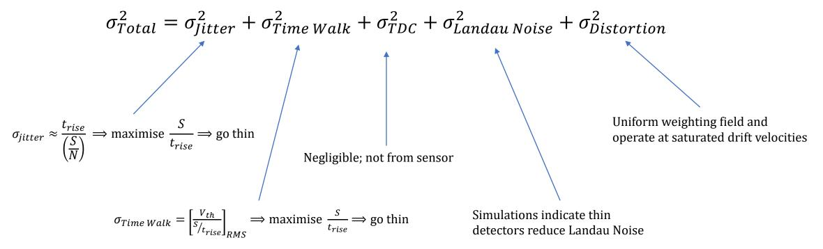
• Best timing resolution obtained by  ${\sim}50 \mu m$  sensor thickness and higher gain of  ${\sim}20$
