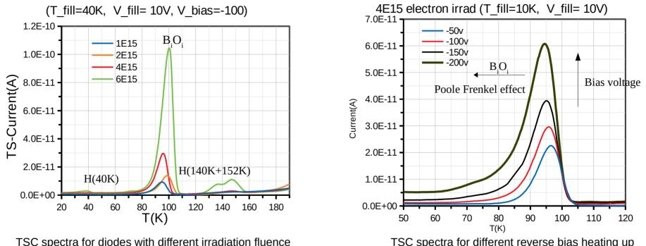
TSC spectra for diodes with different irradiation fluence
