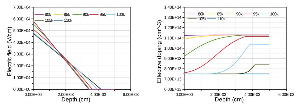
The distribution of electric field and doping profile for different temperatures. During  $B_iO_i$  emission, the changes of electric field and doping profile is observed.
