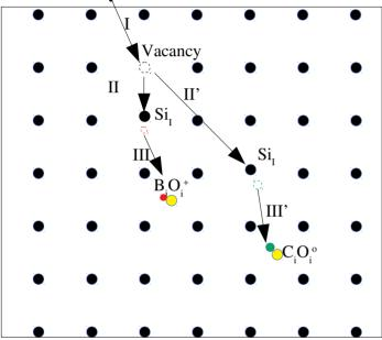
Schematic of radiation damage in p-type silicon material
