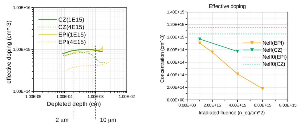
Doping profile for CZ and EPI diodes with fluence 1E15 and 4E15 e/cm<sup>-2</sup>. (left figure)
