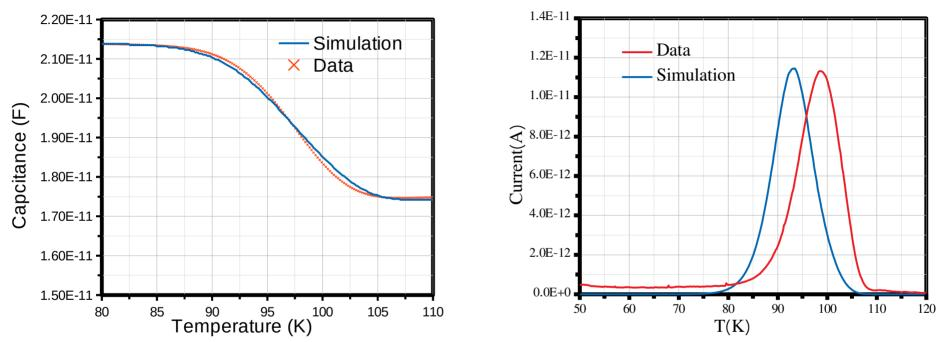
Comparison of simulation and data for TS-Cap (left) and TSC spectrum (right). Possible reasons for the difference between simulation and data:
