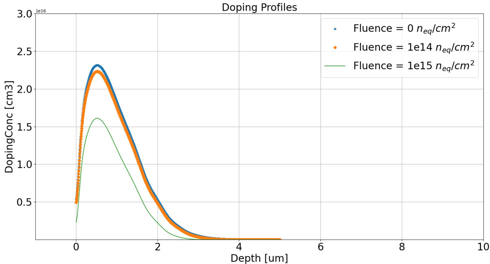
Acceptor removal mechanism
