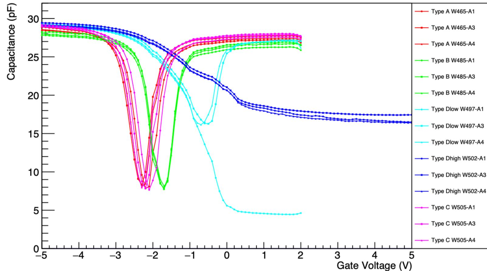
Special Processing GCD - Large Gate -  $V_{diode} = 5V$
