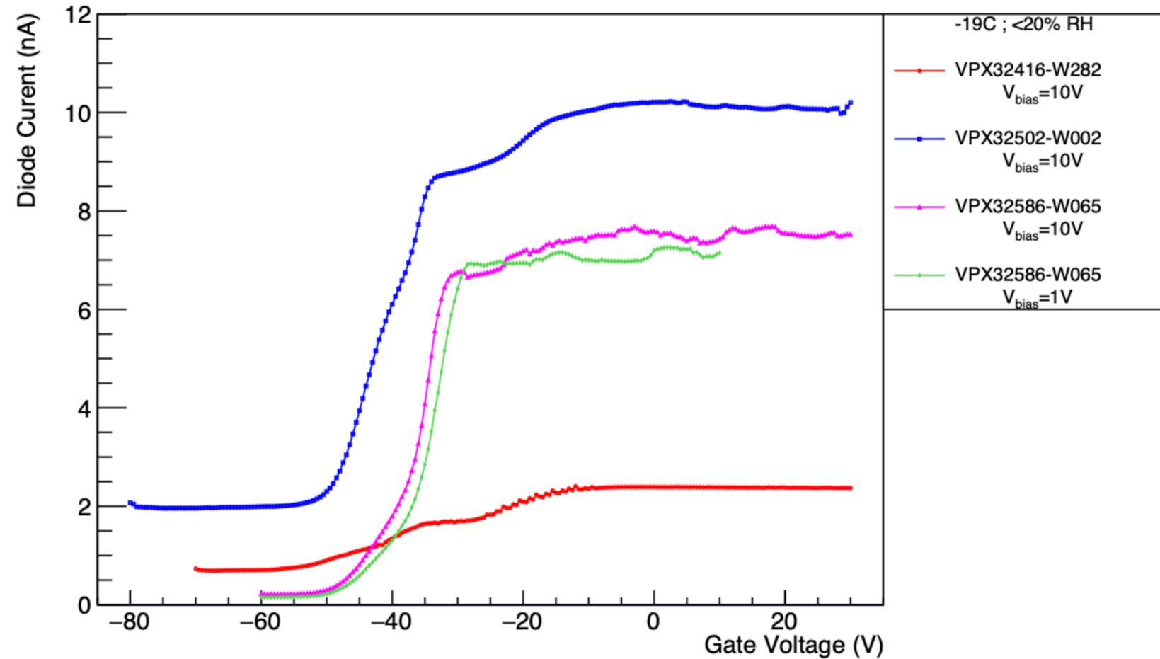
Gamma Irradiated GCD VPX32502-W002
