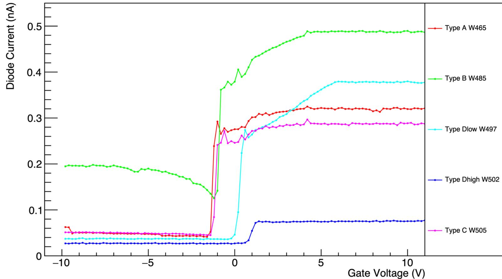
Special Processing GCD - Large Gate -  $V_{\text{diode}} = 5\text{V}$
