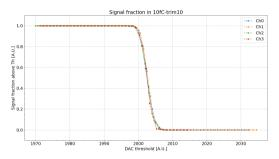
"Handmade" **trimming** by shifting Ch0, Ch1 and Ch3 curves of the distance between the VT50 of Ch2 and the VT50 of the channel, leading to similar response across channels
