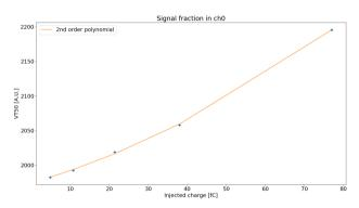
Value of VT50 of Complementary Error function (ERFC) plotted as a function of input charge (5 - 80 fC) for each channel Uncertainty on VT50 position from fit used as error bar in
