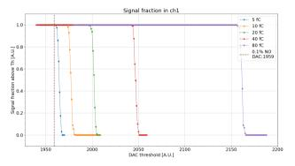
S-curves scan repeated with multiple input charges ( 5 fC, 10 fC, 20 fC, 40 fC and 80 fC) obtained by modulating input signal amplitude (50 - 800 mV)<sup>1</sup>
