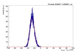
Space resolution reconstructed from difference between laser focusing position (from TCT) and position obtained from  $\chi^2$  minimization (statistically independent data set)
