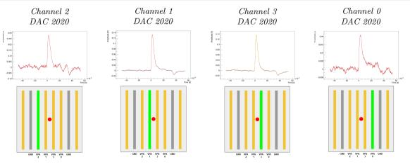
Study of relative signal amplitude on different neighbouring strips can be exploited in reconstruction with **center-of-mass algorithms**
