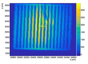
Colour indicates **integral charge of the signal peak** from the ALTIROC analog output
