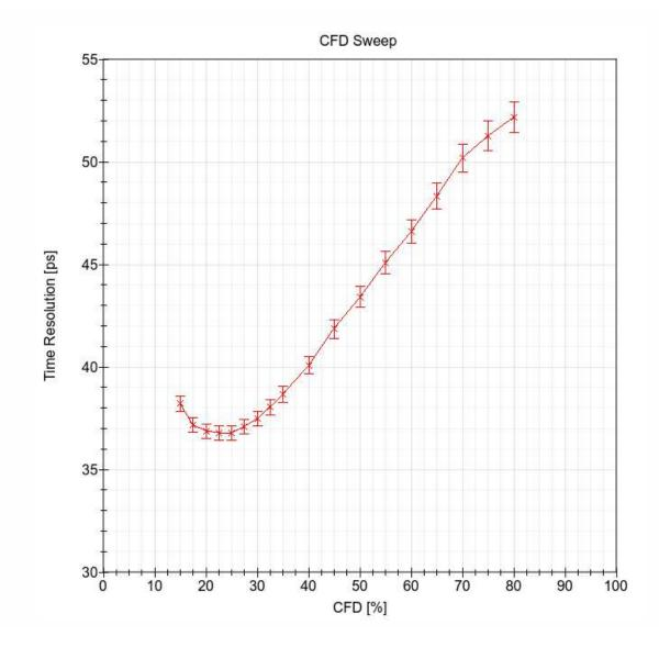
• As mentioned previously, the CFD makes a large impact on the timing resolution (calculated using the factor of root 2). We use a value of 20% (although a value of 25% is often used by others)
