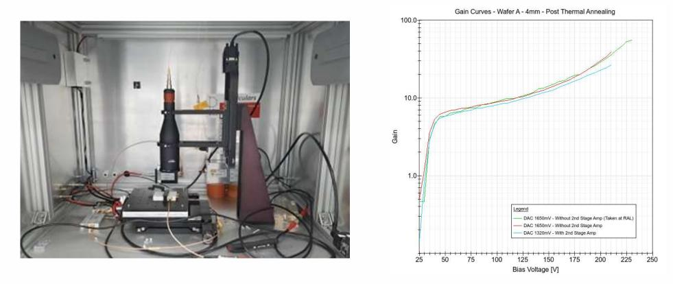
• The gain of our devices can be calculated by injecting charge via a 1064nm IR laser
