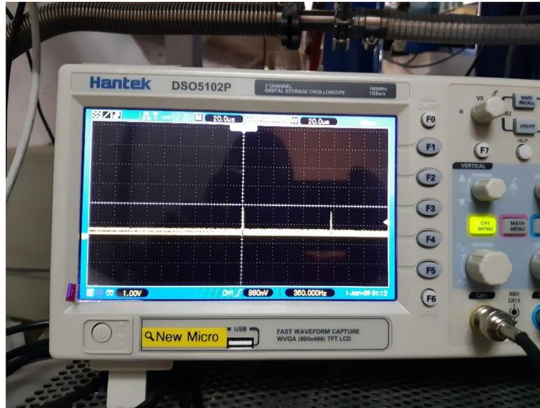
2 MeV Proton Flux control very precise by a local scope looking at the pick up signal
