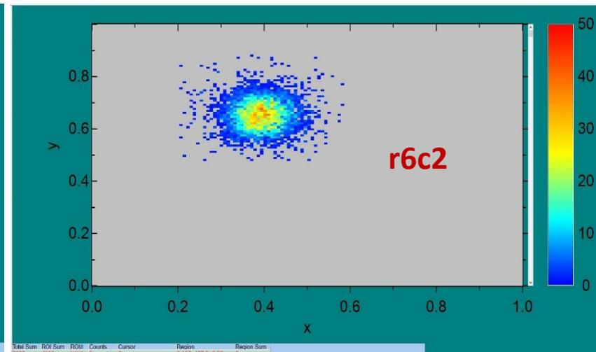
2 MeV 200 protons/sec, 640x640  $\mu\text{m}^2$  zig-zag scan, 60V bias, 30  $\mu\text{m}^2$  spot area
