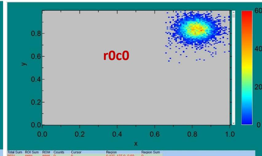
2 MeV 200 protons/sec, 640x640  $\mu\text{m}^2$  zig-zag scan, 60V bias, 30  $\mu\text{m}^2$  spot area
