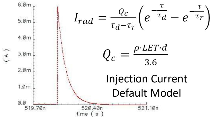
An injection current source at every node or at user selected nodes is the way to emulate the SEE. The injection source model can be changed.
