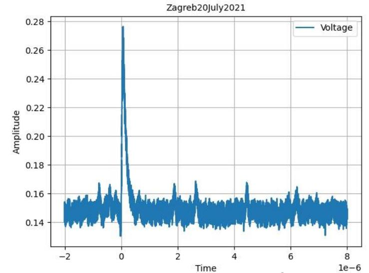
2 MeV 200 protons/sec, 640x640  $\mu\text{m}^2$  zig-zag scan, 60V bias, 30  $\mu\text{m}^2$  spot area
