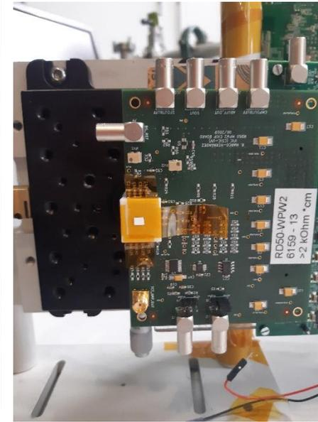
Coarse aiming with a gadolinium scintillator patch
