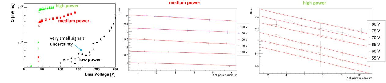
Similar observation as for T3.2 sensor, with even more pronounced gain increase at low density. Problem is large signal for large density and saturation of the amplifier.
