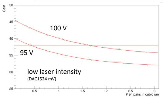
G(95 V, 0.4 e-h/um3)=G(100 V, 1.5 e-h/um3) Higher n<sub>e-h</sub> has to compensate for the difference in "external" electric field:
