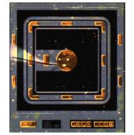
Particulars Scanning-TCT beams spot FWHM~10 μm pulse duration <350 ps 1064 nm light used (660 nm, 520 nm to be used)
