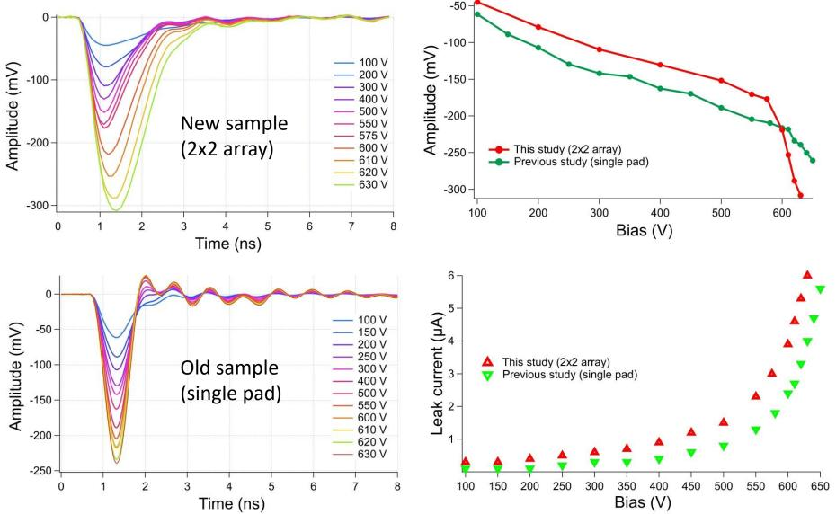
Above 600 V waveforms for new sample are significantly broadened
