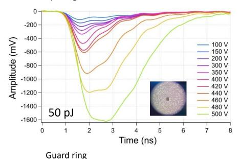
The opening window in FBK sensors are much smaller than in others but still big enough (~10x10 um) to safely focus the beam inside.
