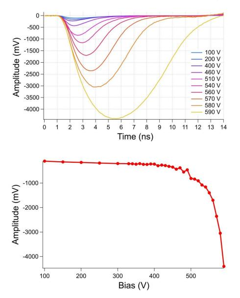
Signal of the sensor vs bias is relatively linear for lower values (up to 400 V). For higher values we observe rapid highly nonlinear increase of the signal amplitude and significant broadening of the waveforms.
