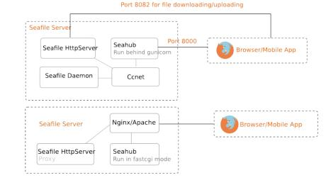
The picture below shows how Seafile mobile client interacts with Seafile server: two opsions - with nginx configure or simple setup
