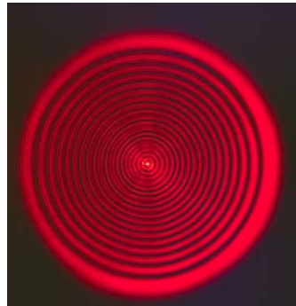
Fig. 4. Structured light beam with almost non-diverging bright central part, useful for optical elements alignment.
