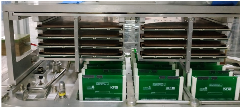
Figure 26: Top plate of the GAP TPC with the 8 FECs mounted and the input adapters plugged in. The Kapton cables are not yet installed.
