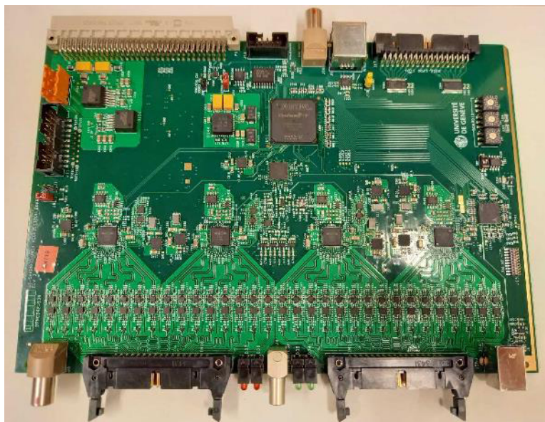
Figure 33: The DRS4 board for PSD read-out.
